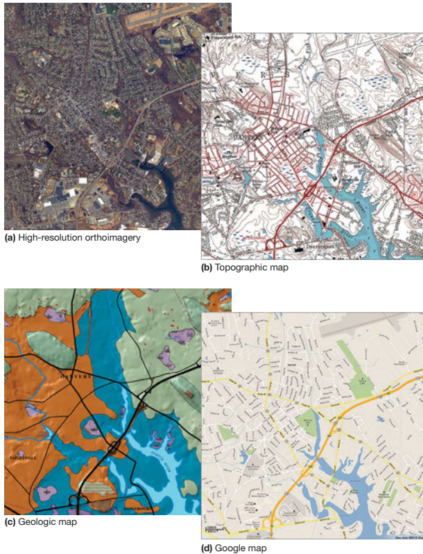
▲ Figure 2-1 Different types of maps convey different kinds of information about the landscape, as shown in these four maps of a region near Salem, Massachusetts. (a) High-resolution orthophoto imagery (original scale 1:24,000). (b) Topographic map with elevation contour lines (original scale 1:24,000). (c) Geologic map showing rock types: orange = coarse glacial deposits; blue = glaciomarine deposits; green = glacial till; lavender = swamp deposits (original scale 1:50,000). (d) Google™ Map showing streets and highways.
